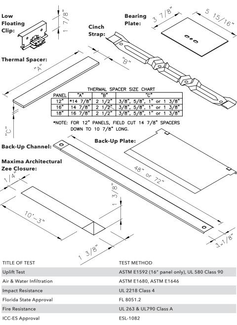
All testing conducted with a Galvolume® substrate.
